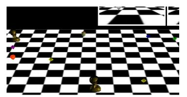
The print below shows the detective camera detection. At this stage, it was possible to observe that the detective was able to detect the jewels and their positions, but not detecting the creature. Detective was wrongly detecting itself also. This was happening due the WS3D version.
